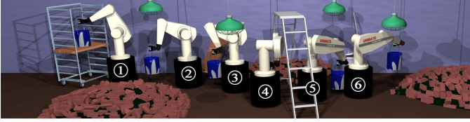
Fig. 10. PAINT: A simulated experiment where the PUMA must transport a can of paint. The plan is required to satisfy a parameterized constraint, C = [0 \ 0 \ 0 \ 1 \ 1 \ 0] , prohibiting rotations about the x and y axes.
