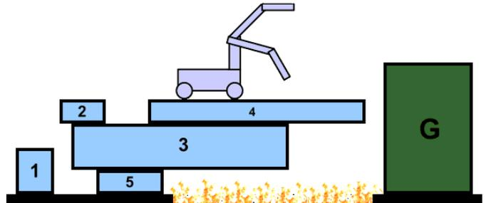
Fig. 1. An example of a robotic agent having designed and built a stable structure to climb the obstacle  $G$  and avoid the hazardous flaming region. Objects  $o_1$ ,  $o_3$  and  $o_5$  have 2 units of mass, where objects  $o_2$  and  $o_4$  have 6 and 3 units. The robot weighs 0.5 unit.
