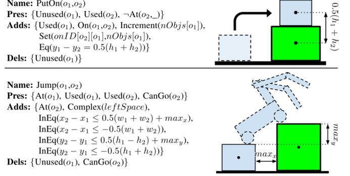
Fig. 2. The example definition for two actions, PutOn( $o_1, o_2$ ) and Jump( $o_1, o_2$ ), which put one object on another and drive the robot over a gap between two objects, along with their effects in the environment.
