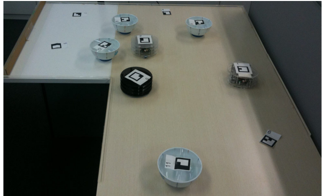
Fig. 1. Multiple robots must push multiple objects to designated goals.
