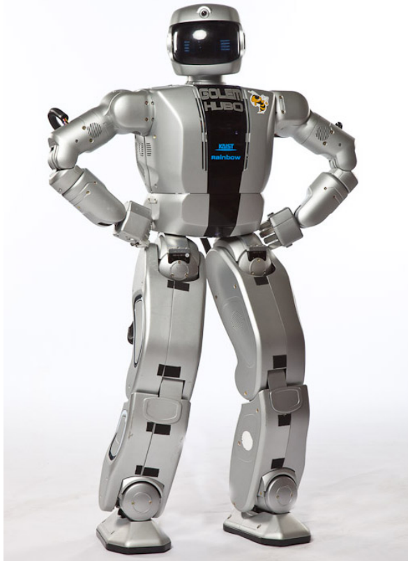
Fig. 1. The Humanoid Robot Hubo2+ for which we calculate kinematics.
