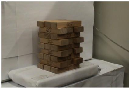
(a) Full tower setup with eight side blocks pulled 0.5cm forward.
